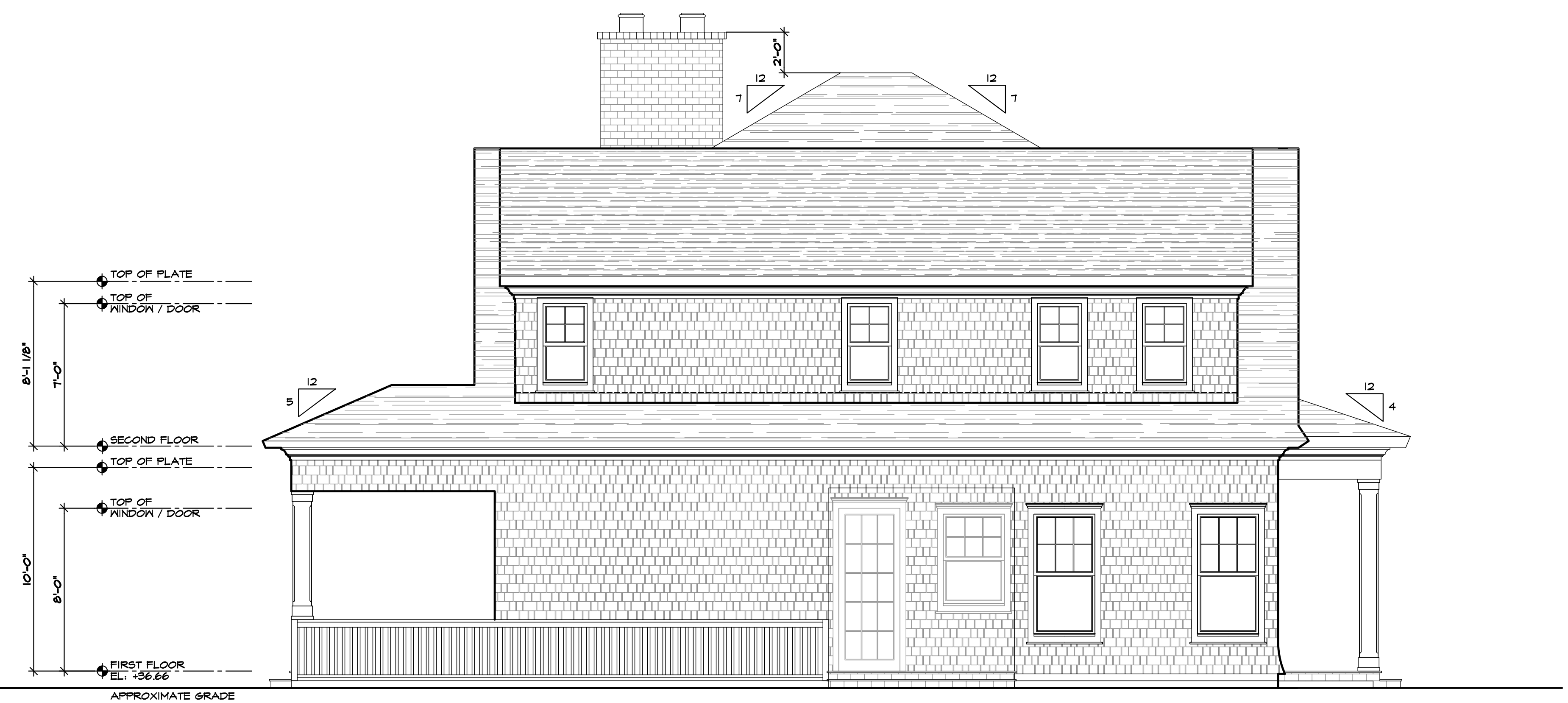
② LEFT SIDE ELEVATION - EAST SCALE: 1/4" = 1'-0"
